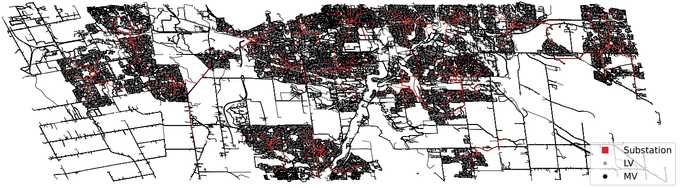
Fig. 3: Synthetic power distribution grid generated for Ottawa city service area. For visualization, the map is rotated by -20^\circ to improve horizontal alignment.
