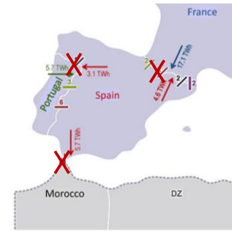
Figure 3. Spain electric grid without interconnection to neighboring systems
