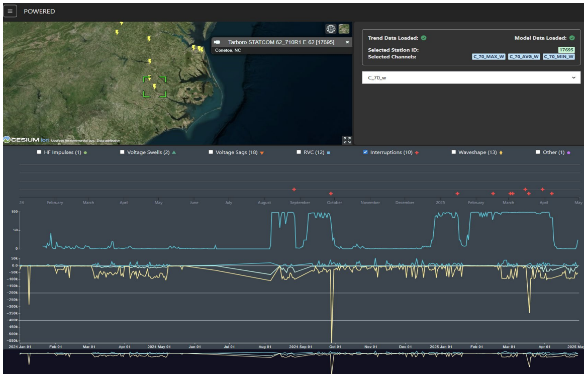
Figure 2: POWERED III interactive dashboard providing geographic visualization of monitored substations (top) with integrated time-series displays of model predictions, trend data, and event histories (bottom).
