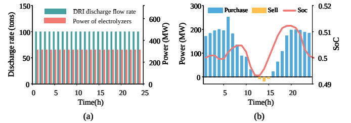
Fig. 4. Operation results of baseline. (a) Discharge flow rate of DRI and power of AE; (b) Purchasing/selling electricity and Soc.
