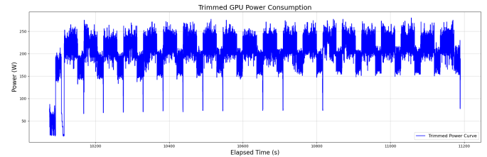
Fig. 1: Power consumption curve of a GPU during the model training of GPT2 124M. Multiple GPUs are synchronized during training, creating volatile and large disturbances on the grid.
