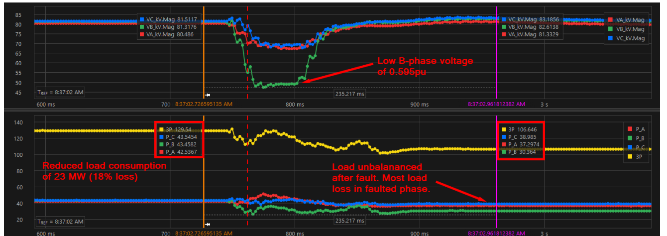
Fig. 1. Voltage and per-phase/total active power of three phases of Facility L at the event of Nov. 18, 2024 [5].
