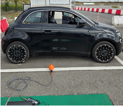
Fig. 1. Fiat 500e used in the measurements and magnetic flux measurement device.
