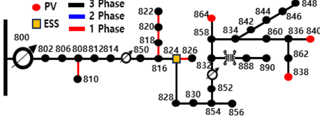
Figure 2. Modified IEEE-34 bus test feeder
