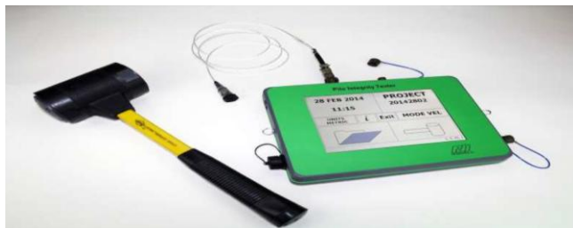
Fig. 7. Apparatus for applying impact and testing
