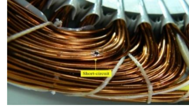
Fig. 1. The equivalent circuit architecture of a three-phase PMSM with a picture of a stator following an ITSC failure in phase a [1].
