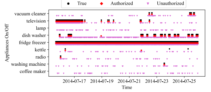
Fig. 3. Inference of on/off state of appliances between noise-adapted (authorized) and standard (unauthorized) FHMM models. \sigma = 1000 W.
