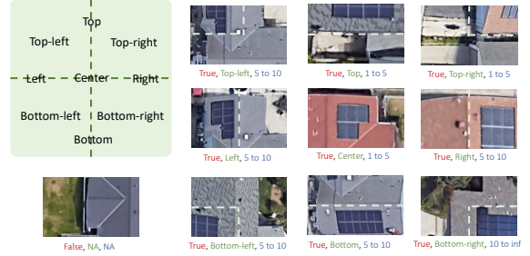
Fig. 2: Solar panel labeling schema and representative examples. The left panel shows nine spatial regions (top, bottom, left, right, center, and four diagonals), plus the “NA” case indicating no solar panels. The right panel displays annotated rooftop tiles with labels specifying (i) presence (True/False), (ii) location, and (iii) quantity range.
