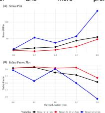
Maximum stress (A) and safety factor (B) versus harvest location. Cortical stress values rise as the harvested bone flap increases in size or is taken more proximally along the medial femoral condyle. Safety factor sharply declines at the largest and most proximally based harvest parameters tested.
