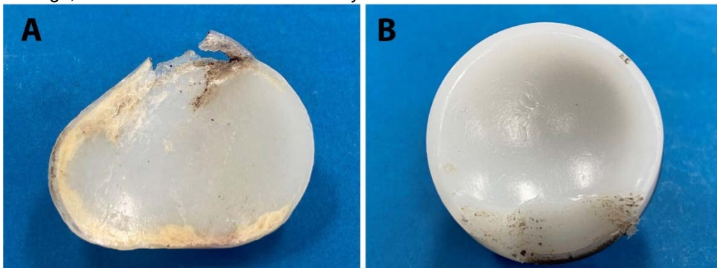
Figure 1A: Severely delaminated aTSA glenoid component with extreme wear-through at rim; B: Excessive rim damage in a rTSA component due to scapular notching which occurs when the PE of the humeral component is in repetitive contact with the inferior scapular neck.
