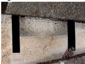
Figure 1. Severe damaged (score 4) to the roughened surface of the hinge on an Apex humeral stem encompassing >75% of the surface. This implant was in situ for 2 years and was removed for pain, dysfunction, and glenoid loosening.
