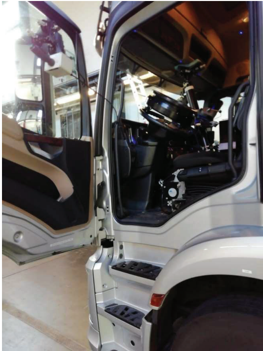
Figure 3: Steering and pedal actuators, mounted in a N 3 tractor vehicle
