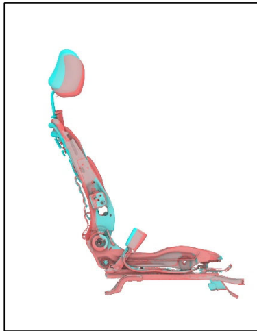
Figure 18: Sled test #2 seat deformation – minimal deformation.
