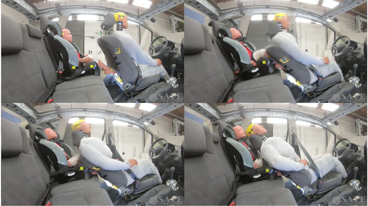
Figure 15: Sled test #1 occupant kinematics – no head-to-head contact.
