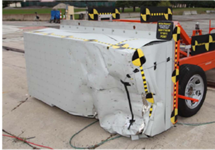
Figure 15 Picture of Full honeycomb crush for the OMDB impacting Mid-size production vehicle
