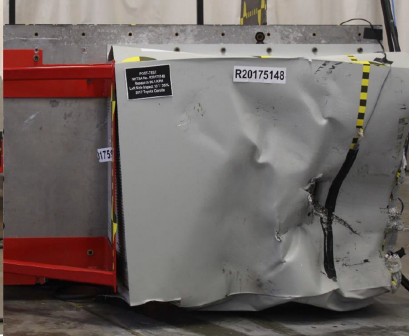
Figure 10 Picture of Half V0 honeycomb crush for the OMDB impacting Small production vehicle *
