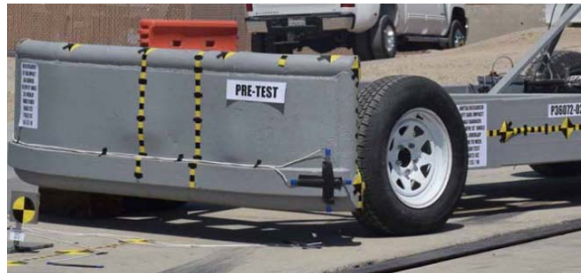
Figure 52 Picture of the moving contoured barrier (MCB)
