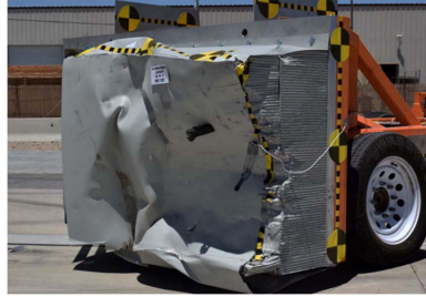
Figure 21 Picture of Half V0 honeycomb crush for the OMDB impacting Large PU production vehicle
