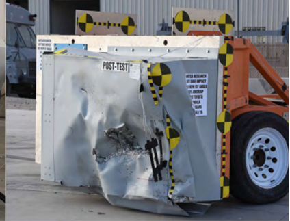
Figure 11 Picture of Half V1 honeycomb crush for the OMDB impacting Small production vehicle
