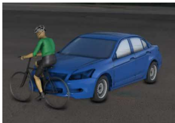
Figure 9. SAFER HBM v9 with helmet on bike impacted by a passenger vehicle travelling at 40km/h.
