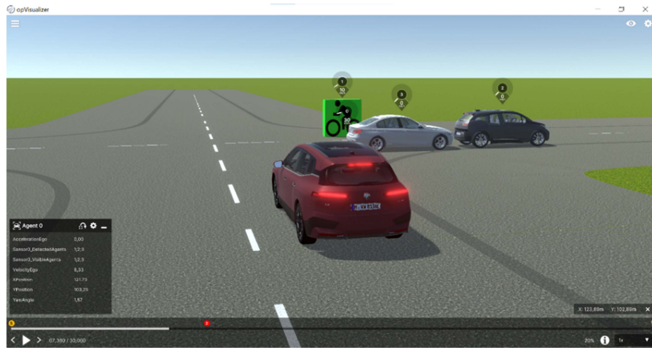
Figure 5: 3D visualization of openPASS simulation in the CBNAO (Car-to-Bicyclists Near Side Adult Obstructed) crossing scenario (ego vehicle: red vehicle).
