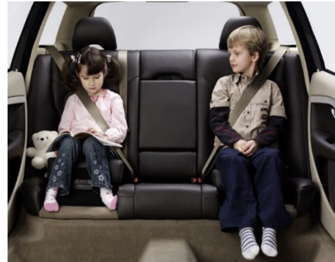
Figure 2c. Two stage integrated booster; high position (left) and low position (right).
