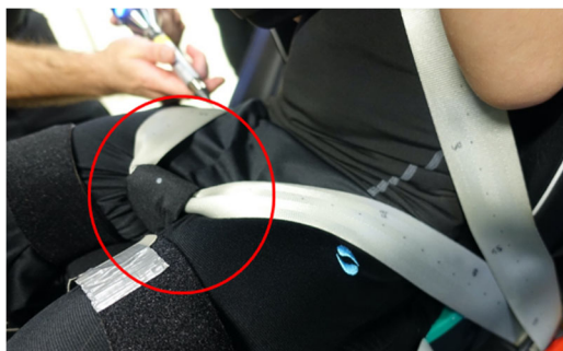
Figure 10c. A child in a booster seat with the lap-belt routed through a lap-belt crotch router strap.
