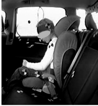
Figure 3a. Maximum forward head position of a child restrained in a booster seat during an emergency braking event (Stockman et al., 2013).
