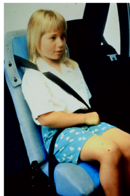
Figure 1b. Early version of a booster seat (1985). The belt guides are of similar design as in Figure 1a, although difficult to see in the photo.
