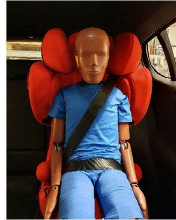
Figure 8c. A booster seat with a 10-year-old-sized ATD in the rear-seat of a modern passenger car
