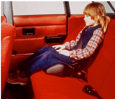
Figure 1a. World-first booster cushion 1978. The belt guides are positioned low on the side of the booster.
