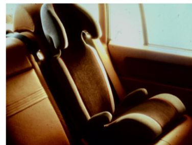
Figure 1c. A booster seat from 1989. As the prior version (Figure 1b), it is a booster seat with removable backrest.
