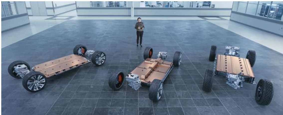
Figure 9: In passenger vehicles, EV battery installations often overlap with occupant compartment footprint
