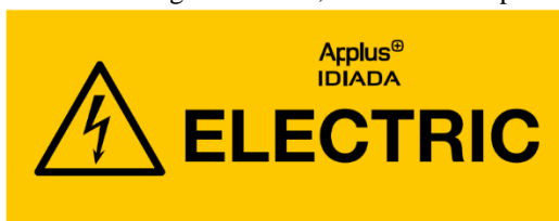
Figure 11: Label used to identify electric vehicles when unloaded into the crash facilities
