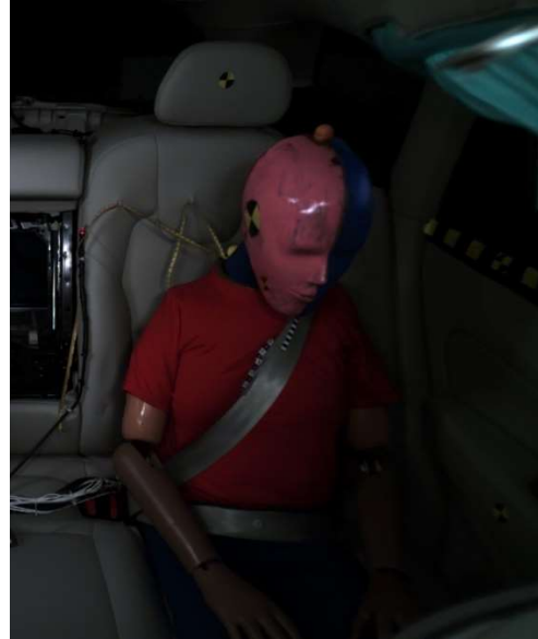
Figure 9b. CF19023 (XC60) belt position after pretensioning
