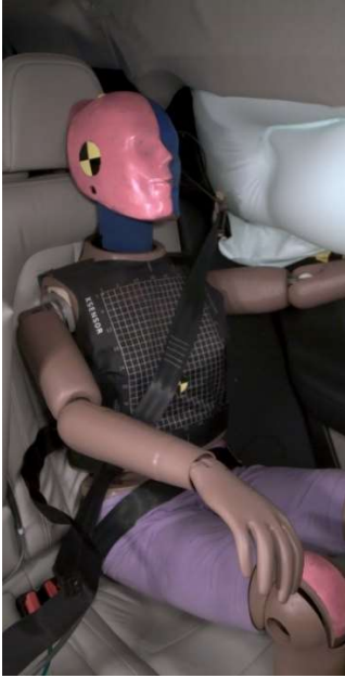
Figure 15a. Stable belt position
