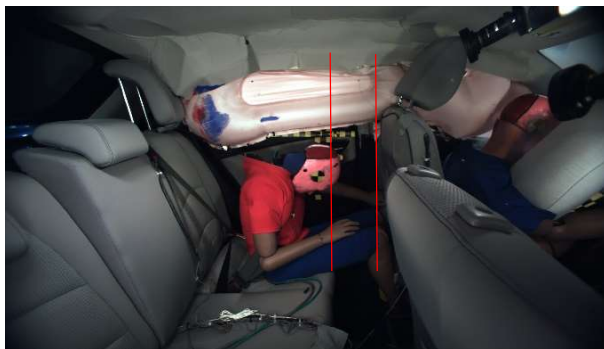
Figure 2b. Photo at 110 ms showing the front seatback moving in phase with the rear-seat occupant's excursion
