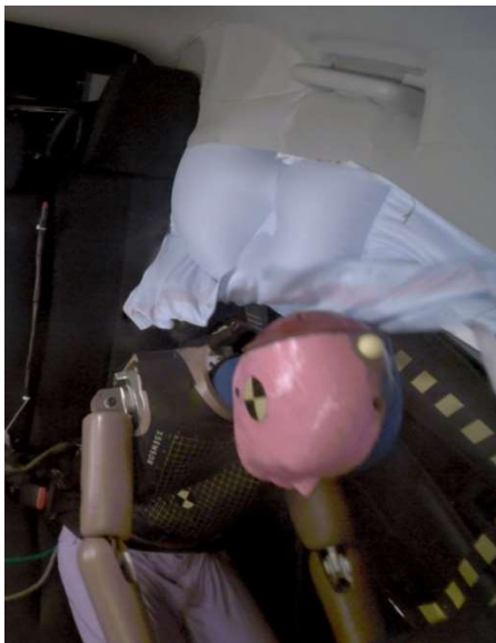
Figure 11a. Lowest dynamic belt position (104 ms); CEP2107 (Eclipse Cross)
