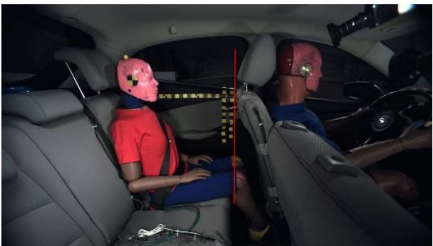
Figure 2a. Pre-impact photo showing the front edge of the vertical tapeline positioned at the rearmost point of the front seatback
