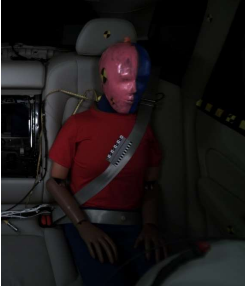
Figure 9a. CF19023 (XC60) Pre-impact belt position
