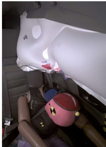
Figure 11b. Highest dynamic belt position (120 ms); CEP2115 (CR-V)
