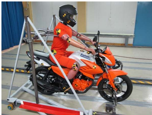
Figure 2. Rider and motorcycle within the frame used to accelerate and launch them to the crash point.
