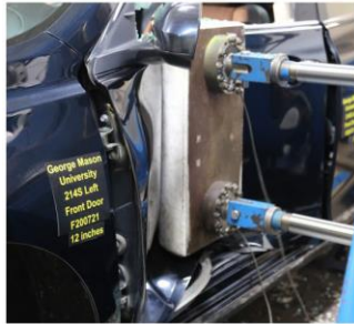
Figure 6. Sedan static door crush test (a) FMVSS 214-static setup; (b) typical force displacement plot; (c) criteria.
